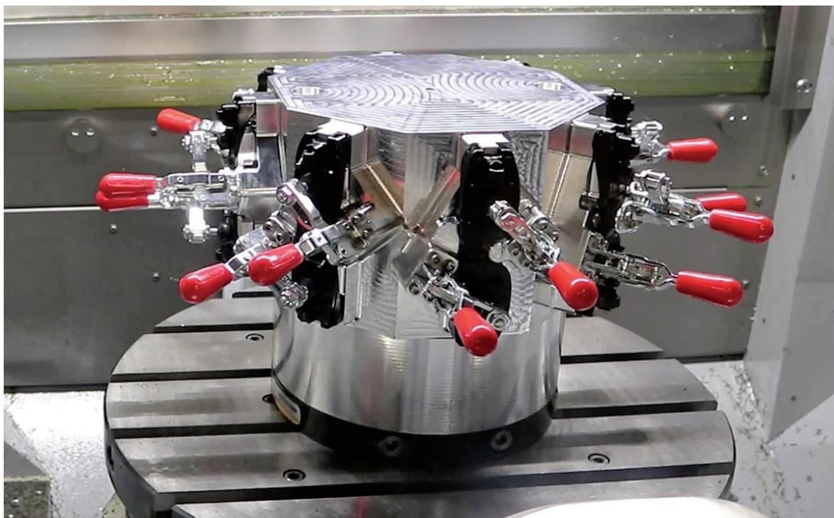
Alpha’s toolmakers also created a unique fixture for a machining step in the process. PolyOne Corp. photo
